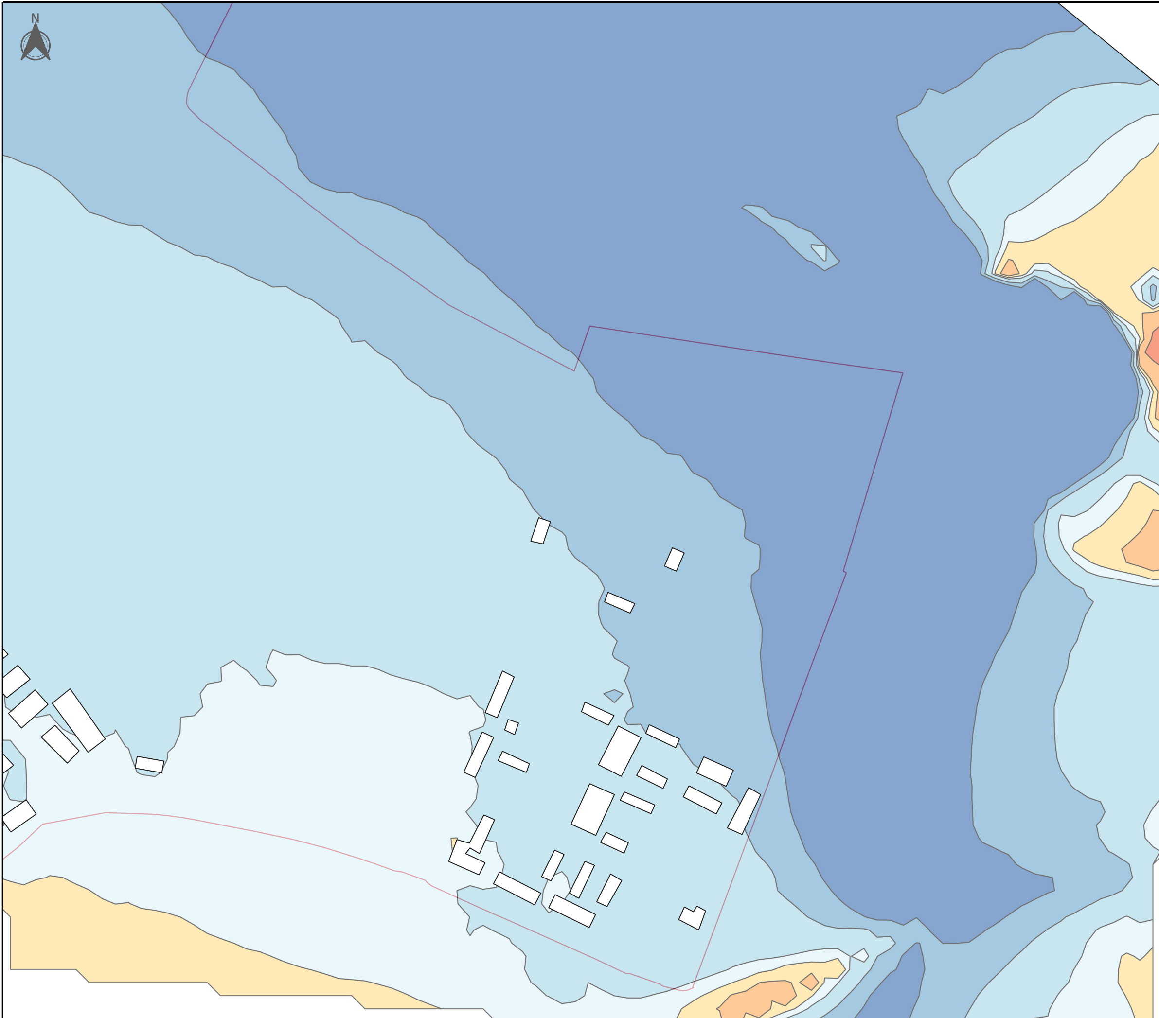
Figure 10.16 Short-term Development Generated Road Traffic Assessment without mitigation - Noise Contours 'difference contours' dB LA10,18h - Grid Height at 1.5m
